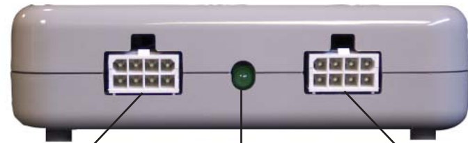
Battery Cable Connection Status Indicator LED Voltage Sense Connection
