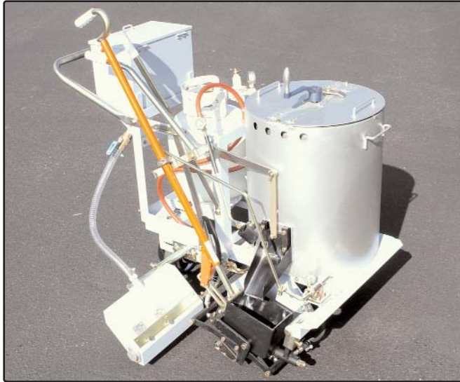
Lightweight material tank is easily removed for quick change of colors.
