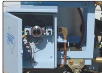
Optional thermostat available for added temperature control.
